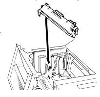
**4** Unpack the toner cartridge from its carton. Hold the toner cartridge with both hands, and shake it well as shown.
